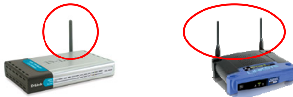
Figure 1. D-Link (left) and Linksys (right) broadband modems with built in wireless access point
